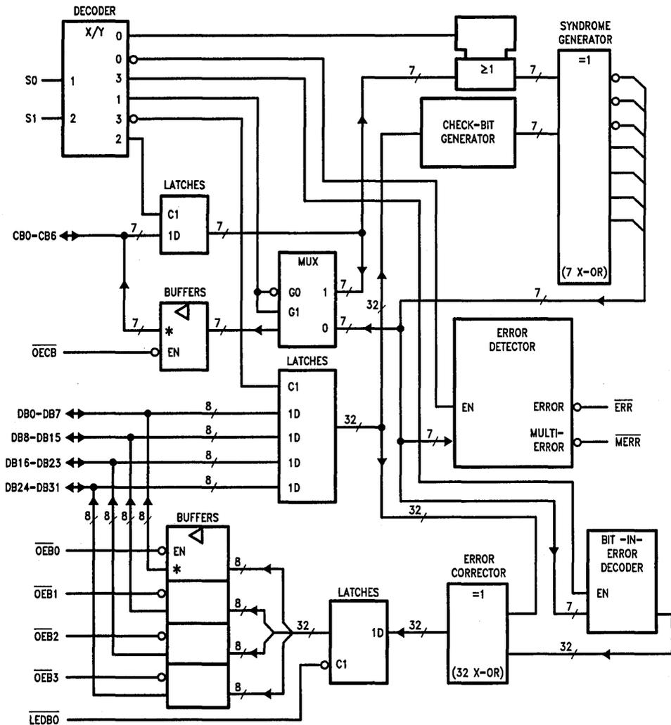
DP8402A HAS TRI-STATE ( $\nabla$ ) CHECK-BIT AND DATA OUTPUTS.
