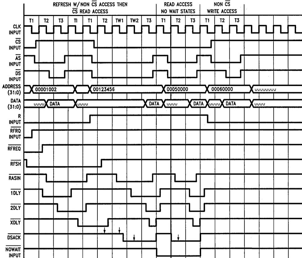
FIGURE 11. System Timing
