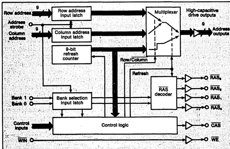
1. Row and column address latches are built into the DP8419 dynamic RAM controller, to meet the needs of microprocessor-based systems that multiplex their data and address lines. The refresh counter keeps track of the next row being refreshed, and a novel addition to any RAM controller, an internal delay line (not shown here), generates the critical access timing on chip.
