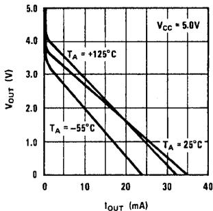
FIGURE 21. Logical "1" Output Voltage vs Source Current
