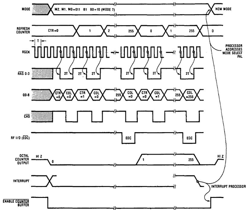
FIGURE 5b. DP8409A All- $\overline{RAS}$  Auto Write Mode, Mode 3a, Timing Waveform
