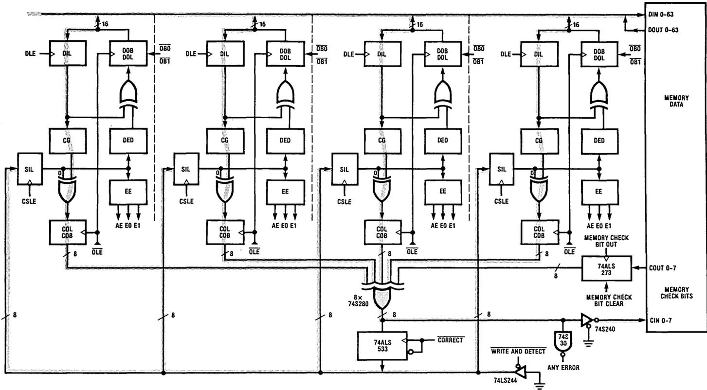
FIGURE 1. E<sup>2</sup>C<sup>2</sup> Simplified Block Diagram—
