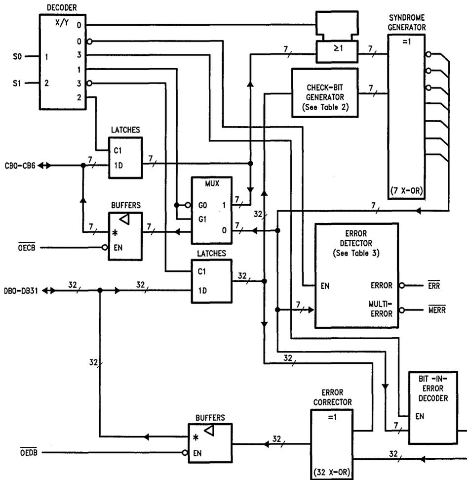
DP8404 HAS TRI-STATE ( $\nabla$ ) CHECK-BIT AND DATA OUTPUTS.
