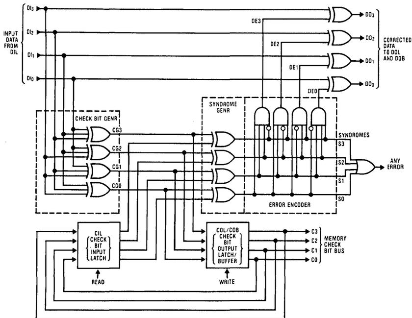
FIGURE 1a. Error Correction 4-Bit Functional Diagram
