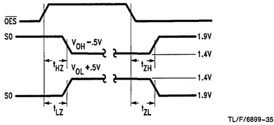
FIGURE 17. TRI-STATE Measurement
