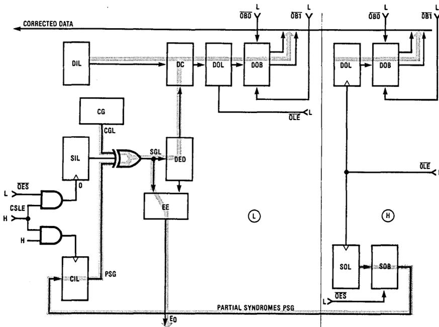
FIGURE 4a. E<sup>2</sup>C<sup>2</sup> 32-Bit Configuration, Error-Correct Flow Path
