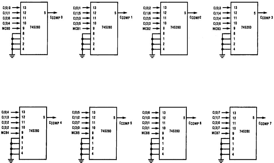
FIGURE 5. E2C2 64-Bit Parallel Expansion
