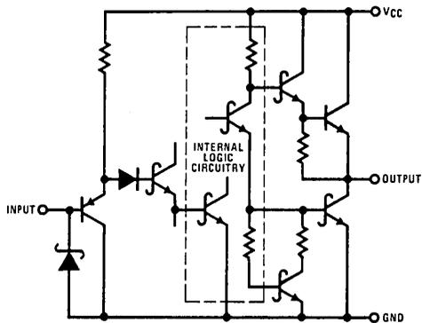
(Equivalent Input/Output Circuit)
