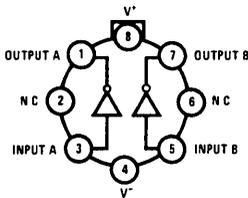
Note: Pin 4 connected to case.
