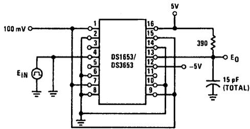
Note: Output of channel B shown under test, other channels are tested similarly.
