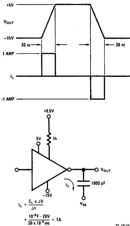
FIGURE 8. Clock Waveforms (Voltage and Current)
