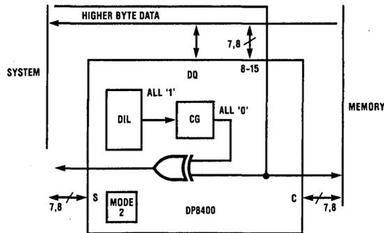
1) DIAGNOSTIC WRITE: WRITE HIGHER DATA BYTE TO CHECK BIT BUS (MODE 2)
