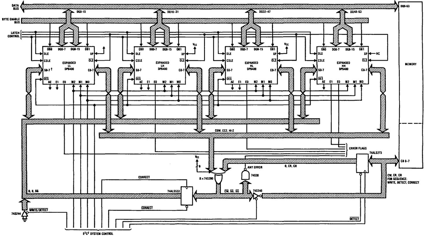
FIGURE 7. Parallel Expansion (Fast 64-Bit Configuration)
