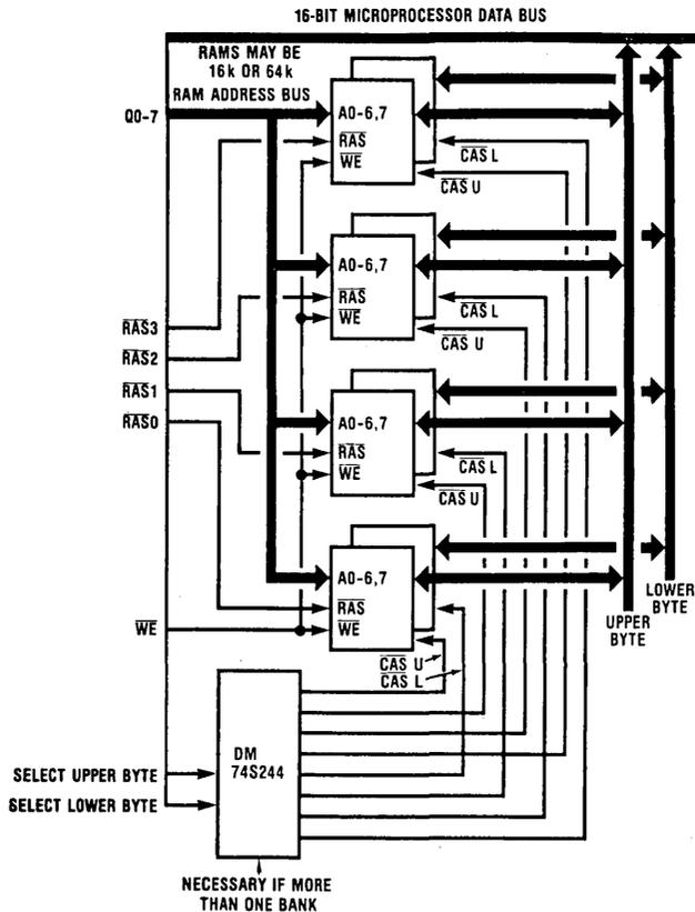
FIGURE 1. Typical 16-Bit Memory with Byte Write Address
