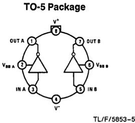
Note: Pin 4 connected to case.
