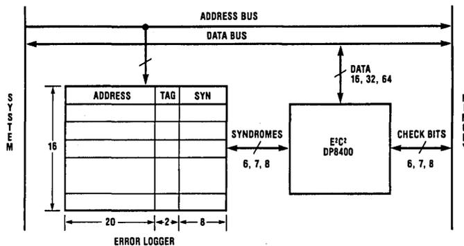
FIGURE 6. Error Logger Connected to DP8400 Syndrome Port
