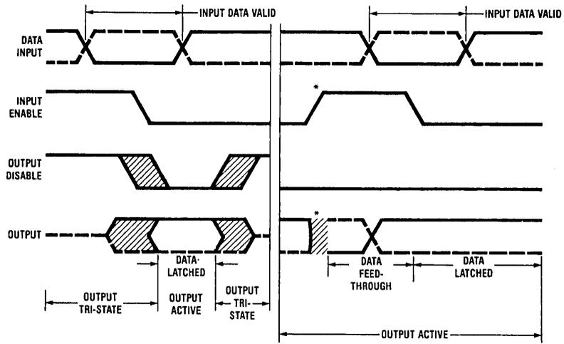
\*When the Input Enable makes a positive transition the output will be indeterminate for a short duration. The positive transition of the Input Enable normally occurs during a don't-care timing state at the output.
