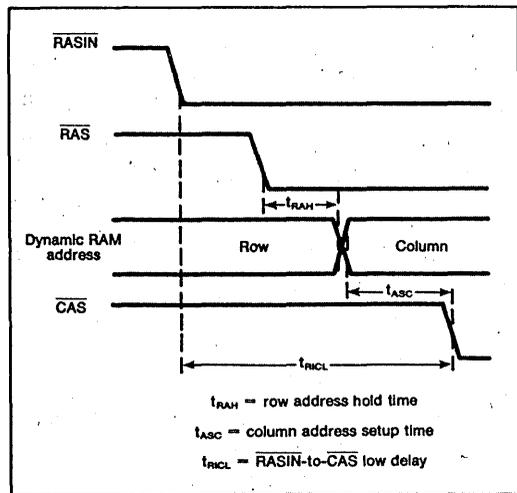
**2. In building a system around dynamic RAMs, designers must focus on the times that the row and column addresses must remain valid,  $t_{\text{RAH}}$  and  $t_{\text{ASC}}$ , respectively. The total delay of the memory controller chip can be defined as  $t_{\text{R1CL}}$ , the delay from RASIN to CAS.**
