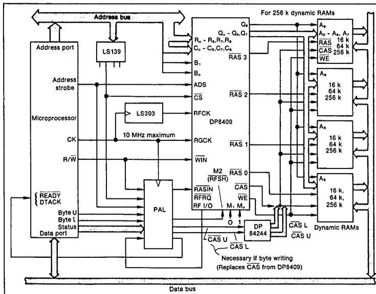
**2. The interface of the DP8409 RAM controller to a 16-bit microprocessor looks ahead to the day when 256-kbit dynamic RAMs are available. By designing-in the controller now, no modifications to printed-circuit boards will be necessary when 256-k devices are developed. Simply exchanging controller chips will allow the memory-control capability of a microprocessor to increase by four times.**
