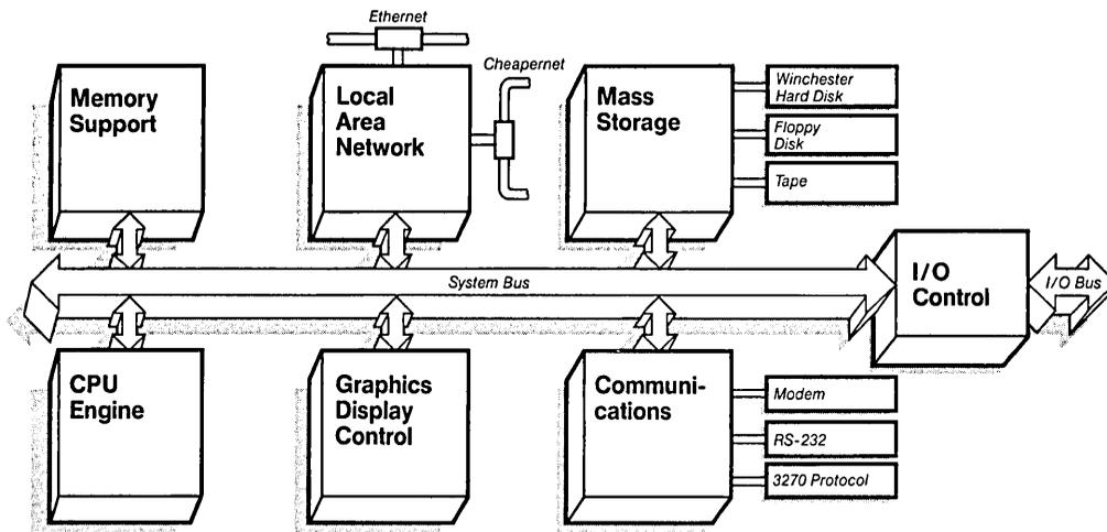
National Semiconductor APPS products include complex VLSI peripheral circuits designed to serve a variety of applications. The APPS products are especially well suited for microcomputer and microprocessor systems such as graphics workstations, personal computers, and many others. National Semiconductor APPS devices are fully described in a series of databooks and handbooks.
