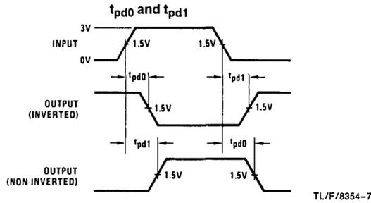
Input Characteristics:  $f = 1 \text{ MHz}$ ,  $t_R = t_F \leq 5 \text{ ns}$  (10% to 90% points), duty cycle = 50%,  $Z_{OUT} = 50 \Omega$
