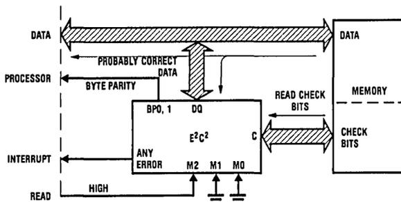
FIGURE 2b. Normal READ Mode, Error Monitoring Method with E<sup>2</sup>C<sup>2</sup>
