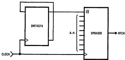
FIGURE 2a. Expansion of Clock Divisor by 2x
