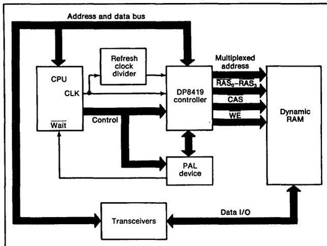
3. In a typical system based on the controller chip, transceivers isolate the dynamic RAM data pins from the CPU data bus. The chief job of the PAL device is to strike a balance between memory refresh and access cycles, and a special divider circuit supplies the controller with one refresh signal per clock period—enough to keep the memory refreshed.
