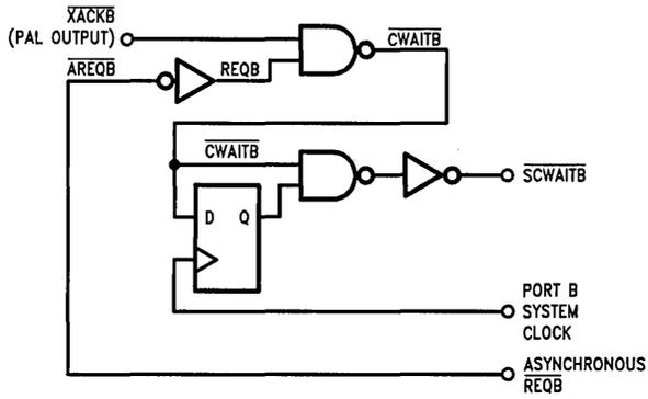
FIGURE 9. Asynchronous Port B transfer acknowledge (" $\overline{XACKB}$ ") synchronizes circuit to produce " $\overline{CWAITB}$ " synchronous with the Port B clock " $\overline{CTTL}$ " (" $\overline{SCWAITB}$ ")
