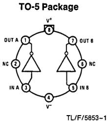
Note: Pin 4 connected to case.
