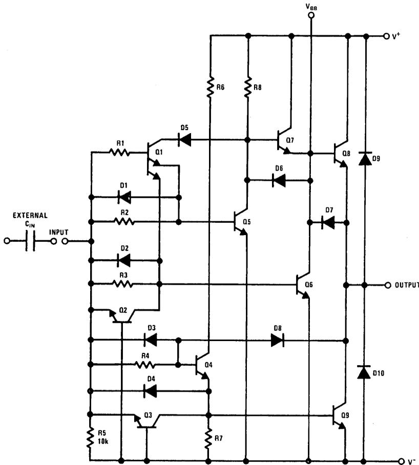
**FIGURE 7. Schematic of 1/2 DS0056**
